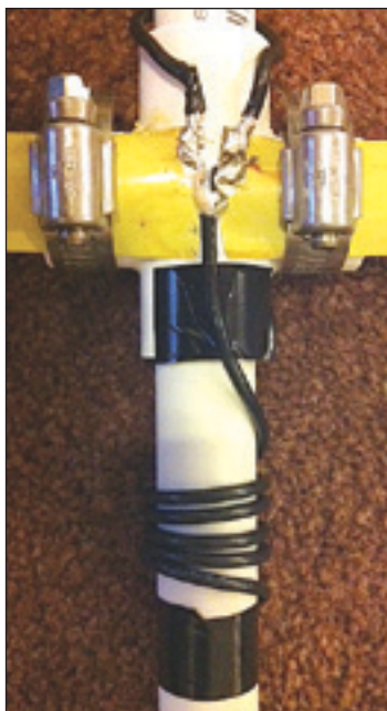
Figure 1 — The director elements can be moved closer in or out to optimize the SWR a little. Don't let them touch.
