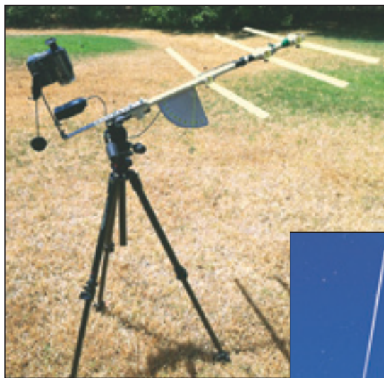
Figure 3 — This is how the setup looks ready for action. A protractor is mounted below the antenna with a washer on a string to “display” the elevation angle. On the left are the handheld transceiver and the camcorder attached to a homebrew mounting bracket. The whole assembly is being held on a standard photo tripod.
