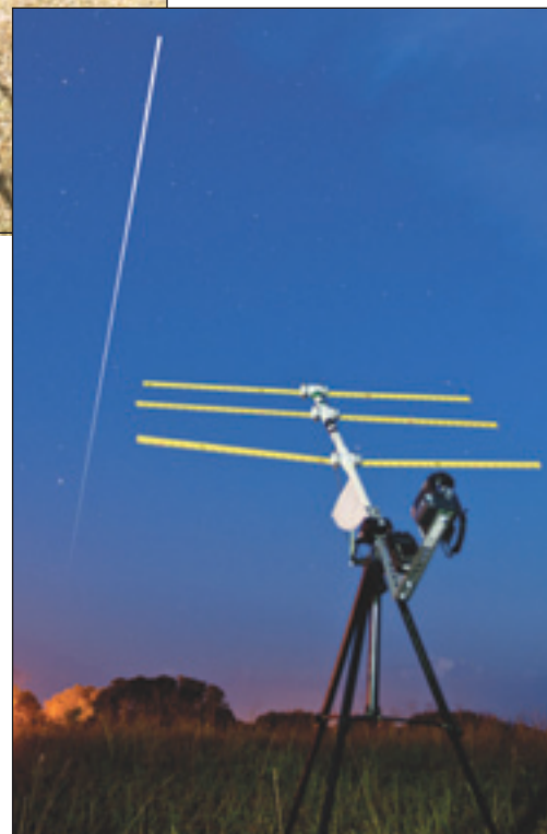
Figure 4 — I took this image on August 10, 2011 from my backyard. In the foreground my tape-measure antenna is set up in position to make contact with the digipeater on the International Space Station, which is traversing the sky leaving a trail in the exposure.
